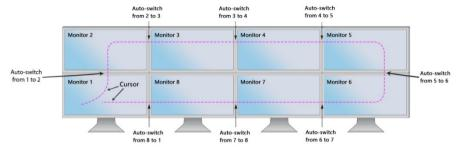
KM0108 automatically switches when the mouse moves between screens.
